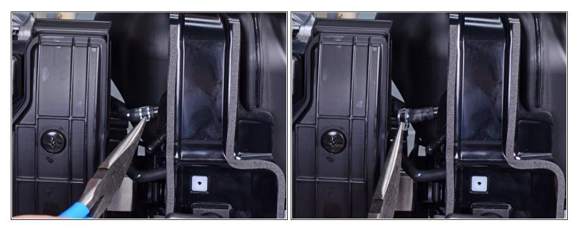
Use a pair of pliers to squeeze and slide the spring clip off the fuel pump port.
