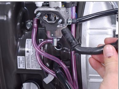
Pull the breather tube straight out of its port.
