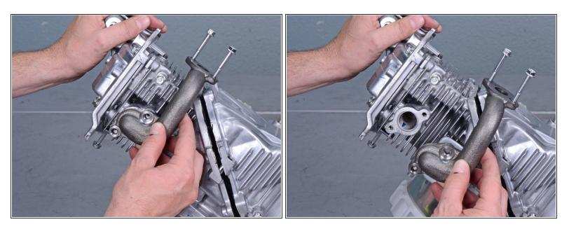
Remove the exhaust pipe from the engine assembly.
