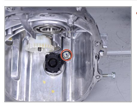
Use a 10 mm socket to remove the bolt securing the oil level sensor.
