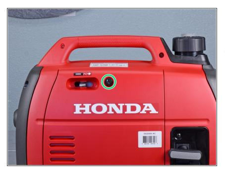
Use a Phillips #2 screwdriver to loosen the screw holding the maintenance cover in place.
