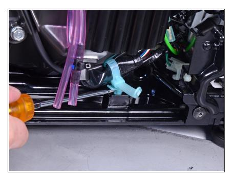
Use a flathead screwdriver to pry up the blue wire harness from the under-cover.
