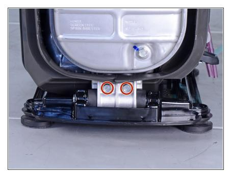
Use a 10 mm socket to remove the two bolts securing the motor rear to the under-cover.
