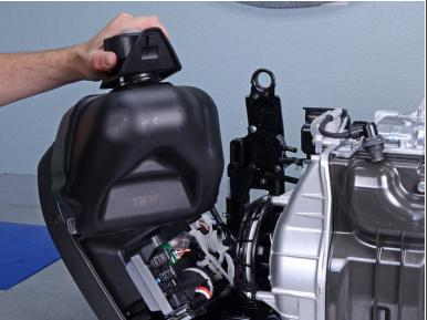
Lift and remove the fuel tank.
