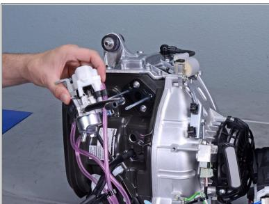
Slide the carburetor off its two bolt rails.
