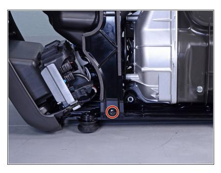
Remove the Phillips screw securing the left (non-access) frame assembly.
