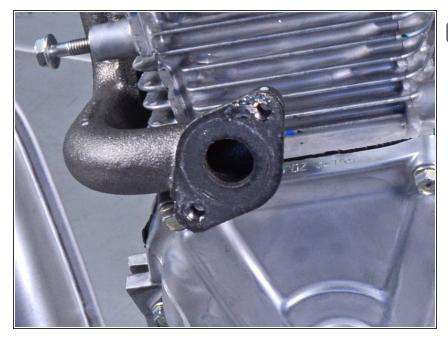
During reassembly, replace the muffler gasket if it shows signs of wear.
