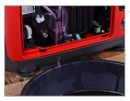
Place a container below the drain tube to catch the excess fuel.
