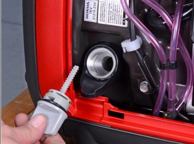
Unscrew and remove the oil filler cap.
