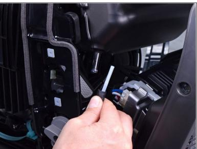
Disconnect the fuel line and filter from the fuel tank.
