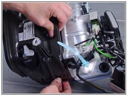
Pull the shroud away along the edge. Use a flathead screwdriver to pry it out of the engine assembly groove.
