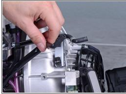
Unclip the fuel and air hoses from the side of the motor assembly.
