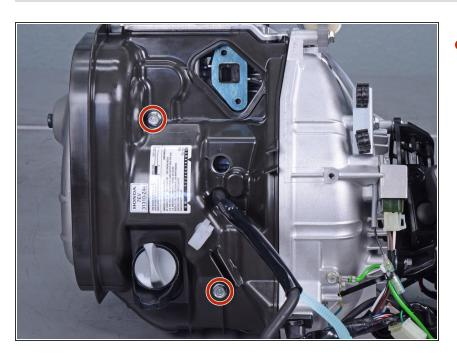
Use a 10 mm socket to remove the bolts securing the right shroud.
