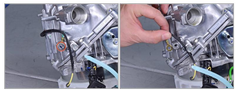
• Use a 10 mm socket to remove the bolt securing the engine oil sensor ground.
