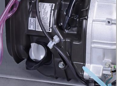
Use a flathead screwdriver to unclip the carburetor wires from the side of the motor assembly.
