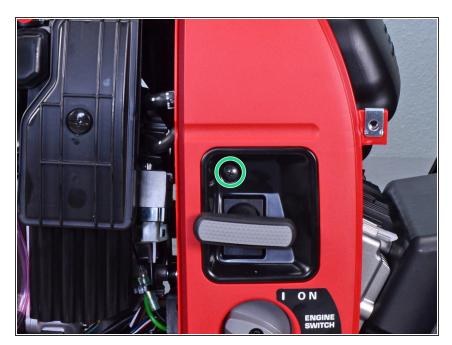
Remove the Phillips screw securing the starter rope port.
