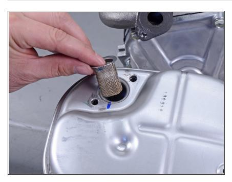
Use a wire brush to clean any deposits off the spark arrester.
