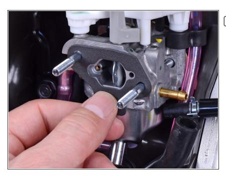
During reassembly, replace the air intake gasket if it shows signs of wear.
