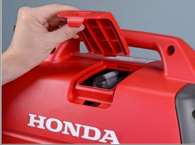
Lift and remove the spark plug cover.
