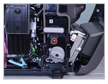
Remove the Phillips screw securing the starter rope guide.
