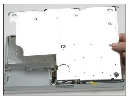
Lift the bottom shield off.
