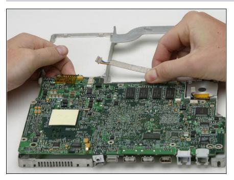
Press the metal framework out as shown and lift the logic board out of the computer, holding it near the battery contacts.
