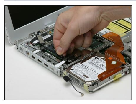
Deroute the display data and microphone cables.
