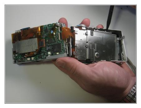
Slide casing out using the spudger.
