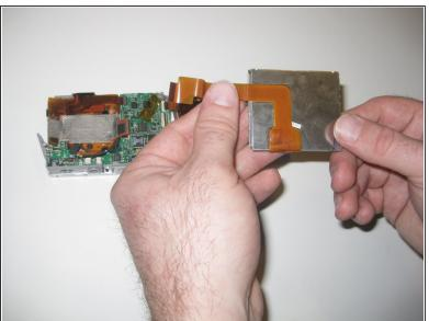
Gently remove the LCD display data cable by gripping the end that is connected to the motherboard and pulling out.
