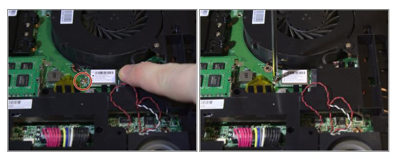
Remove one Philips #0 screw from the motherboard.
