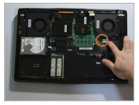
Remove the yellow tape from the wireless card at the center right of the board.
