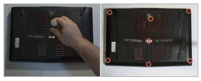
• Remove the seven 6 mm Philips #0 screws on the bottom of the case.
