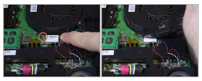
• Using a pair of pliers, remove both wires by pulling straight up from the wireless card.
