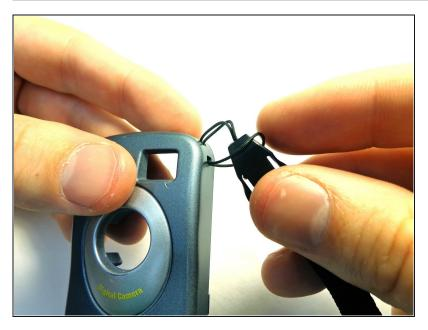
• If the replacement case does not have a wrist strap, remove your device's wrist strap by feeding the plastic tab through the loop cord, and then pulling it all the way through.
