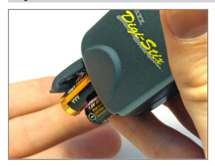
• Tilt device so that batteries slide out.
