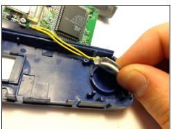
• To remove the microphone from the case, insert the tip of the spudger under the microphone's edge and pry it away from the case.
