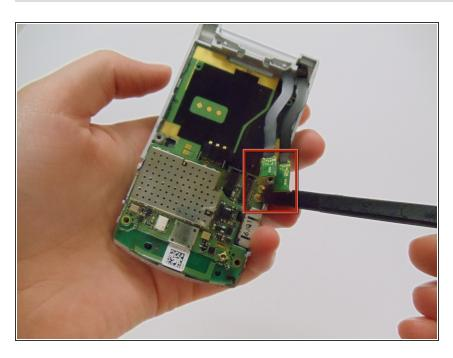
Use the flat end of the spudger to remove two ribbon cables from the back of the motherboard.
