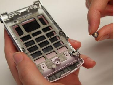
• Use fingers to grab the microphone and remove it from its housing.
