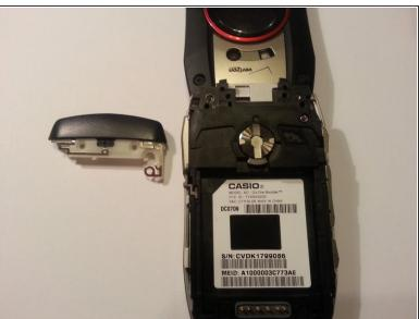
With screw removed, gently pull the antenna outward. It should slide out easily.
