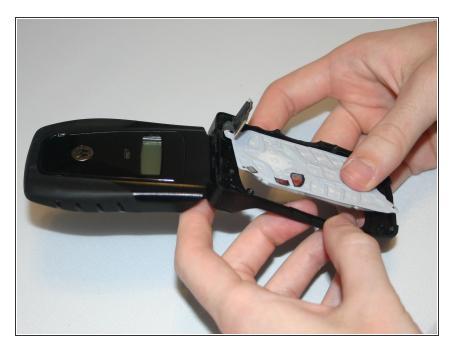
Push lightly from the front of the keypad to remove it.
