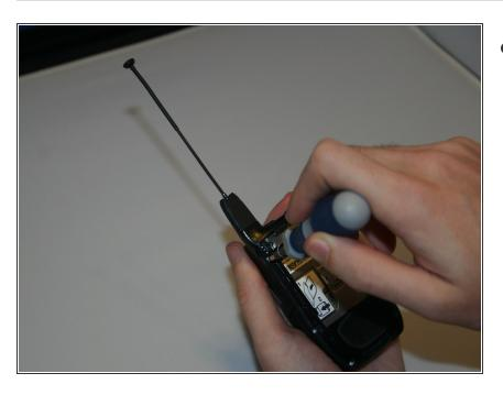
Unscrew all six screws on the back side of the phone using a T-6 bit.
