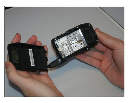
Lift the back panel of the phone to expose battery (not shown here).
