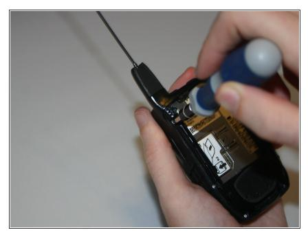
Unscrew all six 5.4 mm screws on the back side of the phone using the T-6 screwdriver bit.
