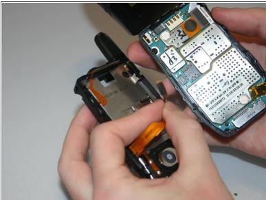
Detach the first ribbon cable by unplugging it from the logic board.
