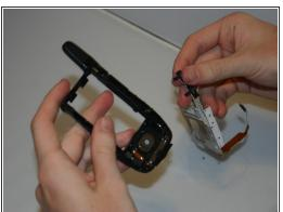
Grab the tab at the bottom of the metal plate, and pull to remove the plate from the phone.
