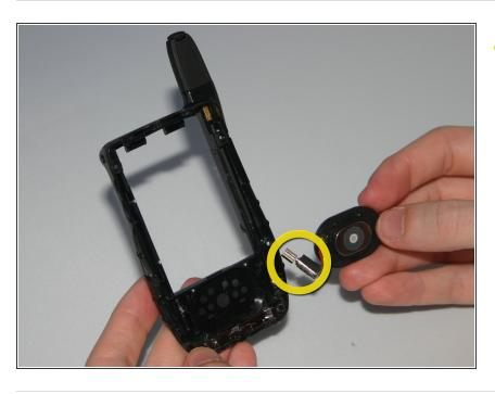
Once the microphone has been removed, remove the connecting piece
