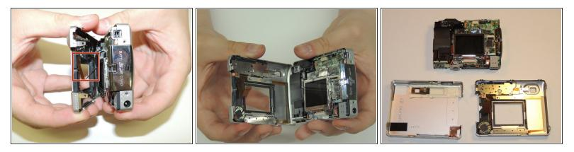
• Then, carefully pry apart the front and back outer casing away from the internal components.
