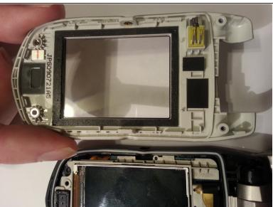
Use a plastic opening tool to remove the screen cover from the rest of the lid.
