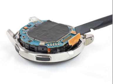
Use a spudger to disconnect the display flex cable from the motherboard.
