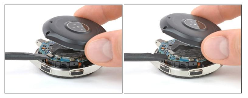
Use a spudger to disconnect the sensor flex cable from the motherboard.
