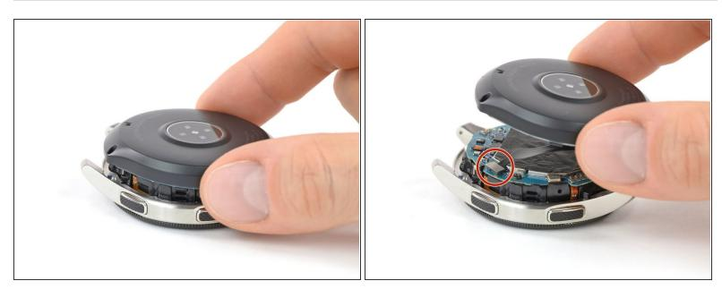
Lay down the watch and lift the back cover to access the sensor connector on the motherboard.
