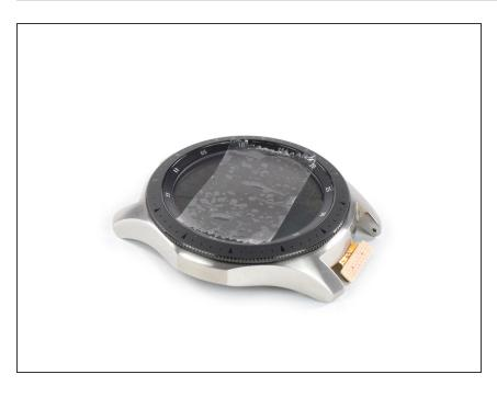
If necessary apply some tape over the display to avoid any injury from glass shards.
