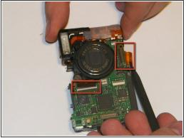
There are two ribbon cables that must be unplugged before removing the assembly. To remove them, simply unsnap the jawbone connectors and then gently pull them out with either the tweezers or the spudger.
