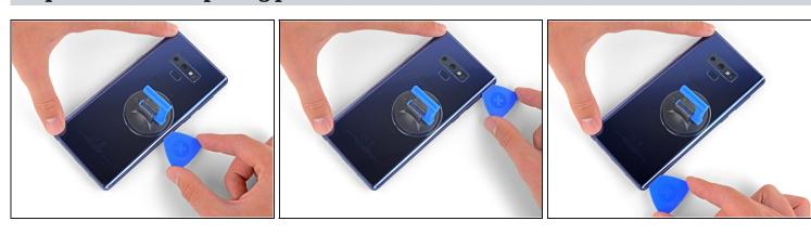
Starting from the center, cut the adhesive up and down the right side with an opening pick.
