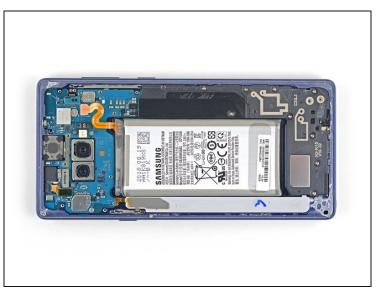
• Remove the nine 4 mm Phillips screws from the plastic cover next to the battery.
