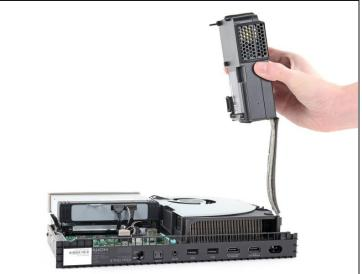
• Lift the power supply so that the cables are at a 90 degree angle.
