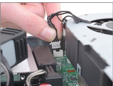
Unplug the bundled cable connector connecting the fan to the motherboard by pulling directly upward.
