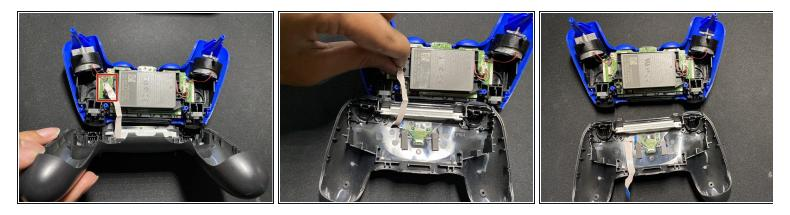
• Unplug the ribbon cable to disconnect the Micro-USB Type B port from the controller itself.
