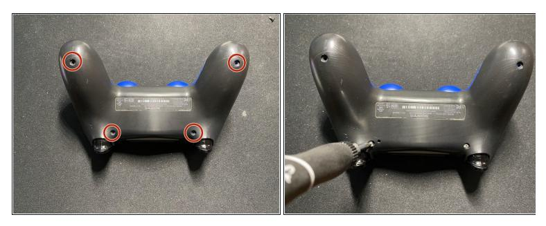
• Connect the front cover and the back cover of the controller and screw the four screws back in.
