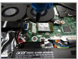
Remove the screw holding down the Wi-Fi card with a Phillips #0 screwdriver.
