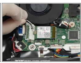
Using your fingers, disconnect the white and black cables connected to the left side of the Wi-fi card.
