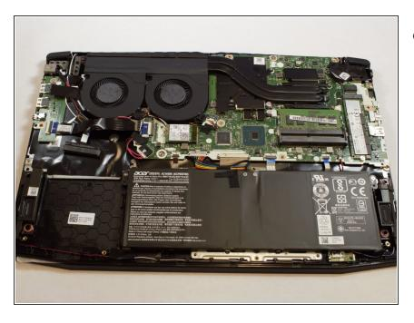
Lift the back cover off once all the clips have been disengaged.
