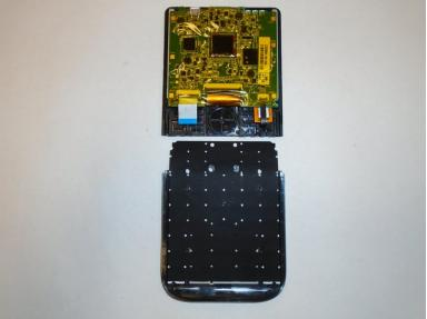
Remove the lower component from the motherboard
