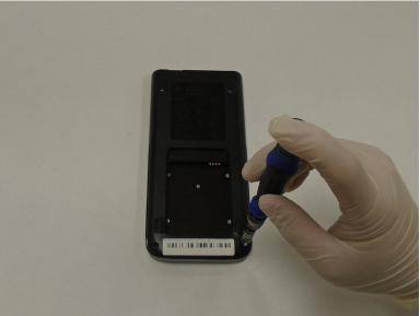
Using a Phillips #00 screwdriver, remove the four 4.5 mm screws securing the back panel to the device.
