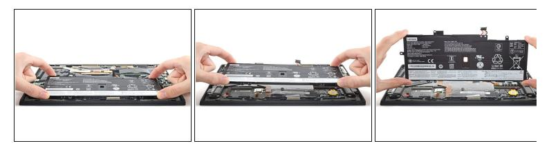
• Lift the battery straight out of its recess and remove it.
