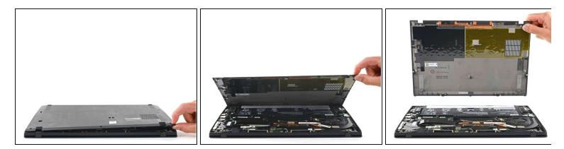
• Lift the back cover up and remove it from the chassis.
