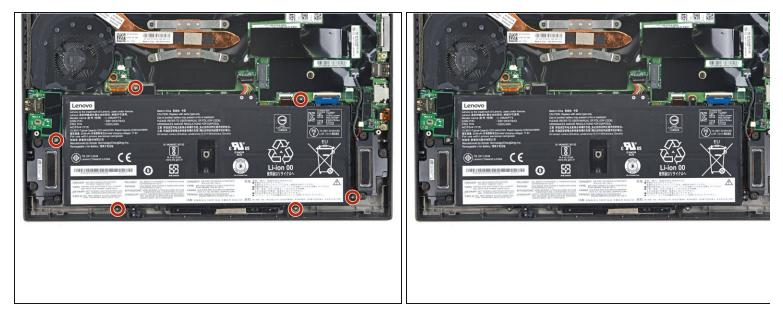
• Use a Phillips #0 screwdriver to remove the six 4.9 mm-long screws securing the battery.
