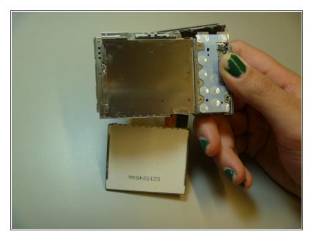
• The LCD is now removed from the camera, although attached by a ribbon at the bottom of the camera.
