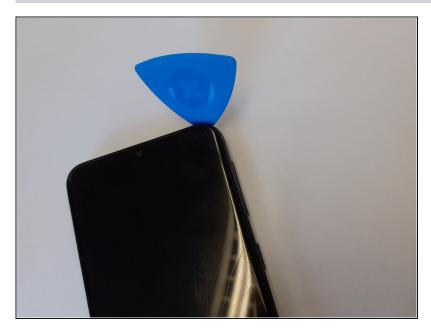
Slide the opening pick from the top left corner to the top right corner to release the plastic clips.
