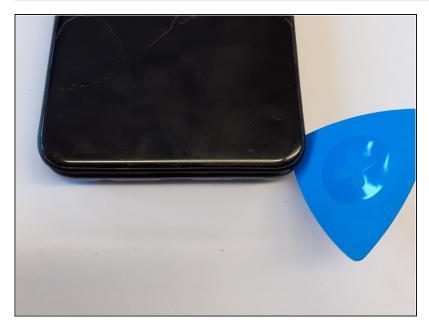
Slide the opening pick from the top right corner to the bottom right corner to release the remaining clips.
