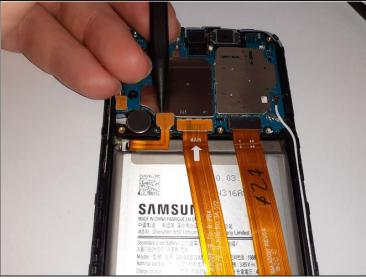
• Use a spudger to disconnect the battery by prying the connector straight up from its socket.
