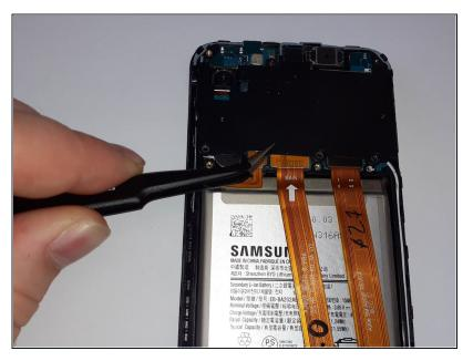
Use the tip of a spudger or tweezers to remove the motherboard cover.
