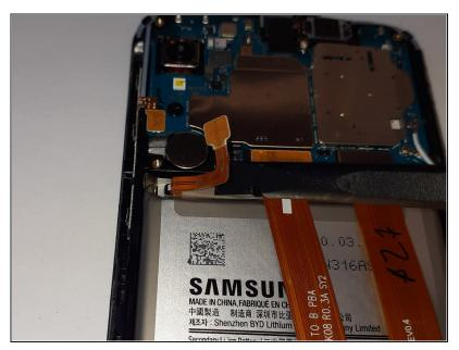
Gently flex the battery connector away from its socket.
