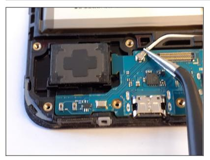
Using a pair of tweezers, gently disconnect the other antenna connector.
