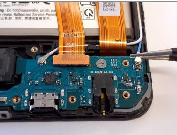
• Using a pair of tweezers, gently disconnect one of the antenna connectors.
