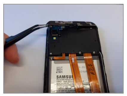
Use the tip of a spudger or tweezers to remove the antenna cover.
