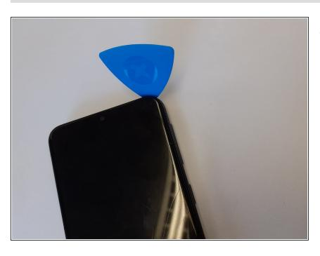
Slide the opening pick from the top left corner to the top right corner to release the plastic clips.
