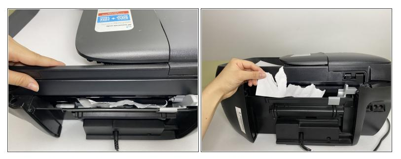
• Check the input tray, located in the back of the printer, for any paper remains and remove them.
