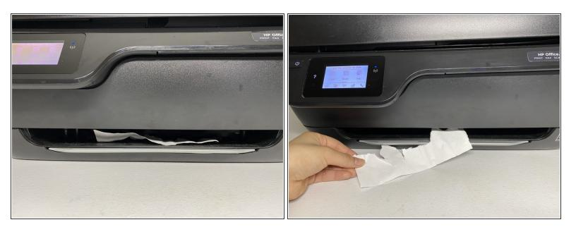
• Check the output tray, located in the front of the printer, for paper remains and remove them.
