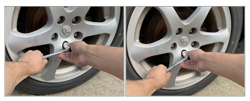
• Unscrew the socket using the socket wrench.
