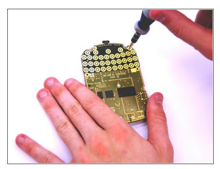
Use a Torx T6 screwdriver to remove the 3 1/8 inch screws shown.
