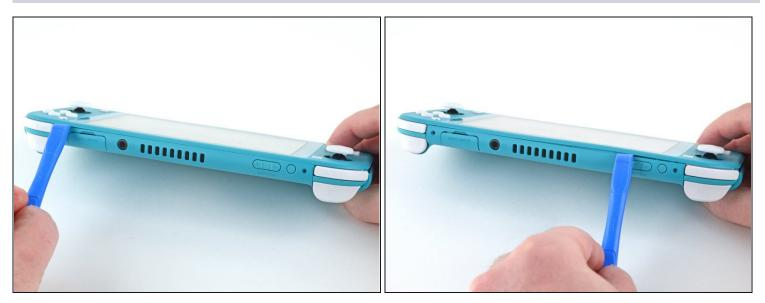
• Continue sliding and prying the opening tool along the gap on the top of the device to release the clips.
