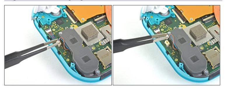
• Use a pair of tweezers or your fingers to pull the right speaker cable straight up and out of its socket on the motherboard.
