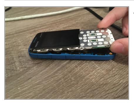
Lift up the logic board / display and remove it from the case.
