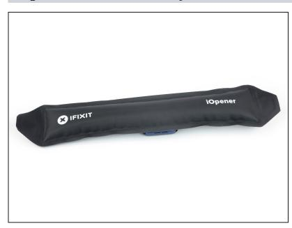
Prepare an iOpener (or use a hair dryer or heat gun) and heat the rear side of the watch to loosen the battery adhesive. Leave the iOpener on the watch for at least two minutes.
