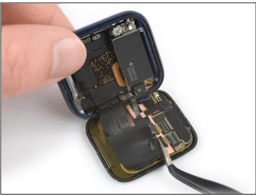
Use a pair of tweezers to pull both display cables out of the ZIF connectors.
