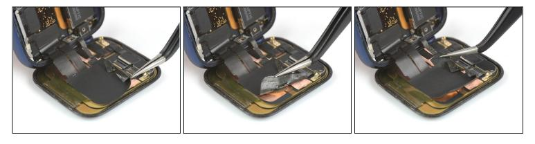
• Use a pair of tweezers to carefully peel off the edges of the sticker which adheres the display and the grounding cable to the rear side of the screen.
