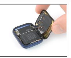
$\triangle$  Be careful not to strain the display cables when you fold the display to the side.
