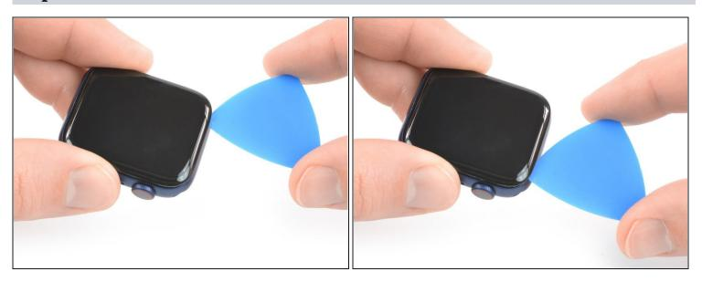
• Slide the opening pick around the corner to cut the remaining adhesive on the short edge of the watch next to the watch crown.
