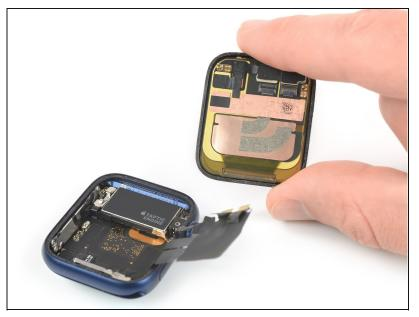
• Separate the watch assembly and the screen.
