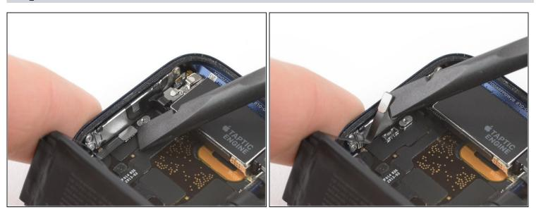
• Use the flat end of a spudger to pry up and disconnect the battery connector.
