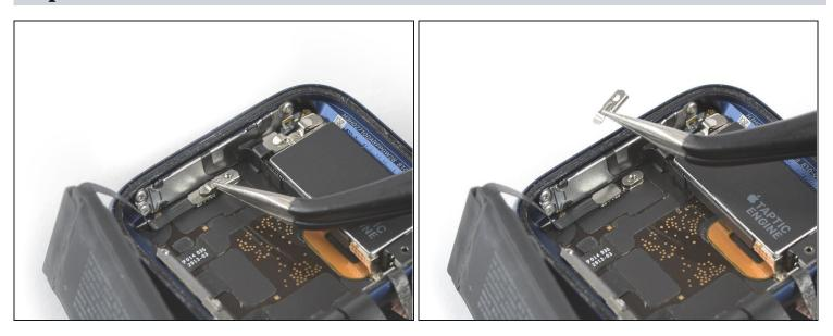
• Use a pair of <u>tweezers</u> to remove the metal shield covering the battery connector.
