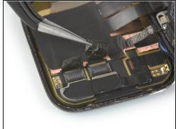
• Use a pair of <u>tweezers</u> to carefully peel the black protective tape off both display connectors.
