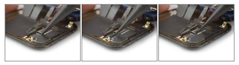
• Use the pointed end of a spudger to pry up the lock bars on both ZIF connectors securing the display cables.
