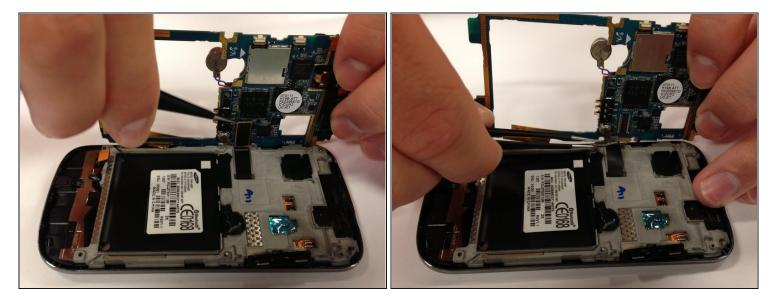
⚠ DO NOT remove the motherboard completely. One more clip on the motherboard's backside needs to be removed.
