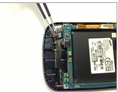
On the right from the lever, use the tweezers to unclip the black connector.
