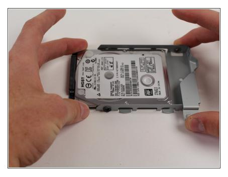
• Remove the hard drive from the sleeve.
