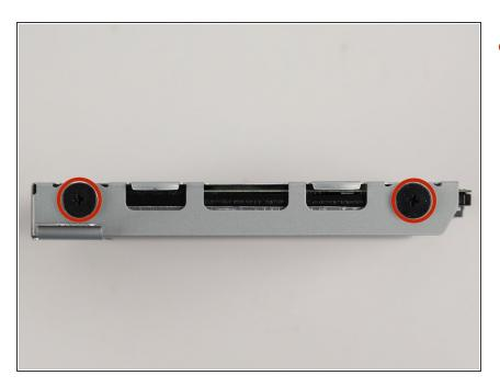
Remove the four screws from the sides of the hard drive case. There are two identical screws on the opposite side.
