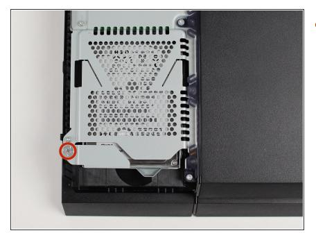
Remove the Hard Drive by unscrewing the single 5mm Phillips head #1 screw on the front left side of the PS4.
