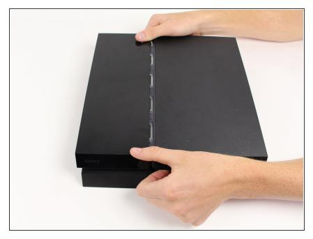
Start by turning off your PS4 and unplugging the AC power cord. Slide the HDD bay cover (the top left portion of the console) to the left.
