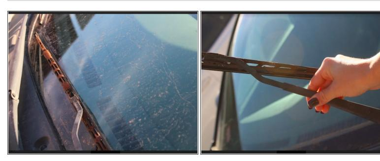
Carefully lift the wiper blade off the windshield of the car.
