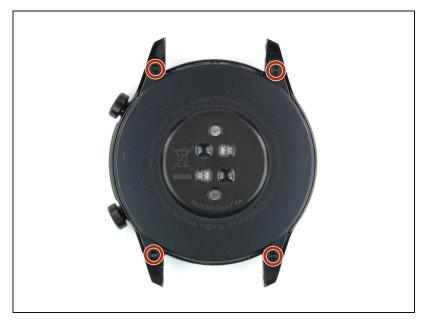
• Remove the four 3.7 mm-long Torx T2 screws.
