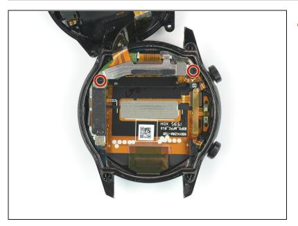
Remove the two 2.3 mm-long Phillips #00 screws.
