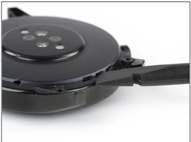
• Insert the edge of a spudger into the middle loudspeaker opening at the top edge of your watch.
