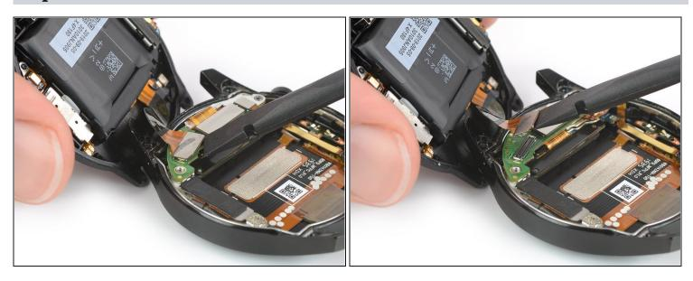
• Use the flat end of a spudger to pry up and disconnect the multi-purpose flex connector.
