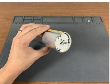
Remove the four Phillips head screws that fasten the motor hub to the tube adapter.
