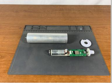
Using a flathead screwdriver, pry the bearing cap from the tube.
