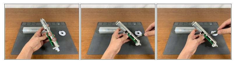
Use a #1 Phillips head screwdriver to loosen the PCB mounting screws until the circuit board can be adjusted. This should only take 1-2 full rotations of the screwdriver. Do not fully remove the screws.
