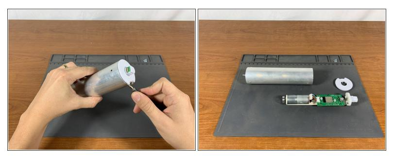
• Using a flathead screwdriver, pry the bearing cap from the tube.
