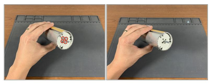
• Remove the four Phillips head screws that fasten the motor hub to the tube adapter.
