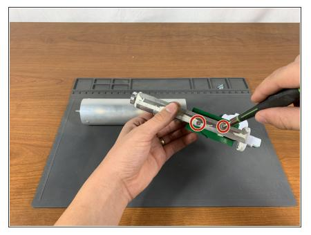
Tighten the two PCB mounting screws until the PCB cannot move freely.
