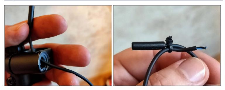
A Push the the whole break/bell part over the handle. And thread the new cable through the hole, as you can see in the picture.
