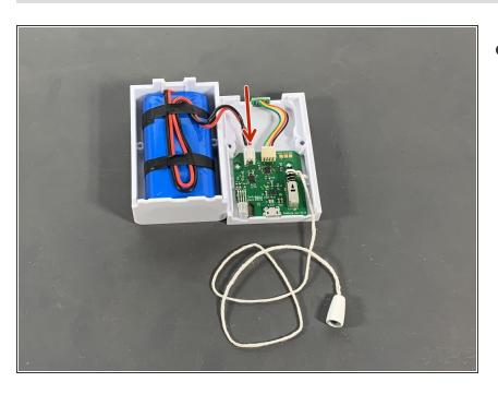
After a few seconds, reconnect the battery pack to the circuit board.
