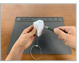
Remove the two Phillips plastic threading screws with a #1 Phillips head screwdriver.
