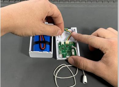
Disconnect the battery pack connector.
