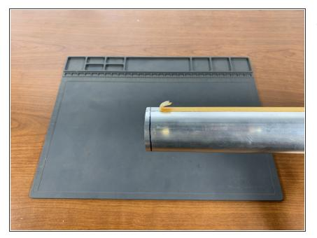
Use a sander, hacksaw, or appropriate metal cutoff saw to shorten the tube to the desired length. Be sure to use the required safety procedures for your chosen method.
