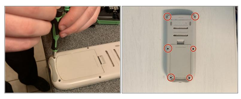
Unscrew all six 8.5mm screws in the back of the calculator using the T6 star screw bit.
