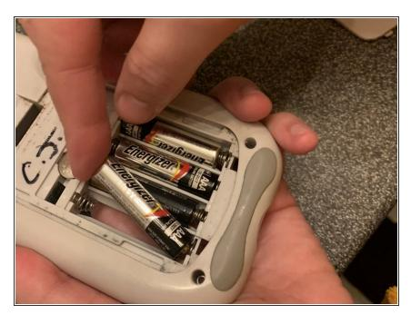
Remove the battery in order to access the battery spring that needs to be replaced.
