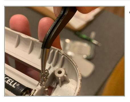
Remove the damaged spring using the tweezers.
