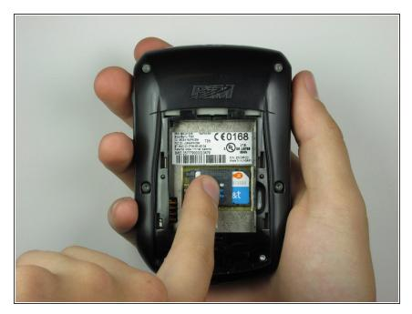
Slide the SIM card holder to the left to unlock the SIM card.
