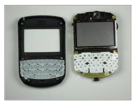
Turn the internals over to reveal the LCD display.
