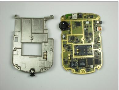
Separate the logic board mounting plate from the logic board by lifting with minimal force.
