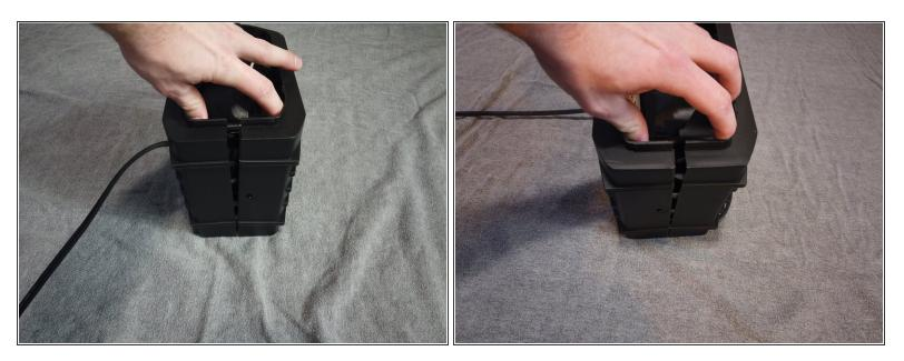
• Use your hands to pry apart the plastic halves of the heater to see the internals of the device.
