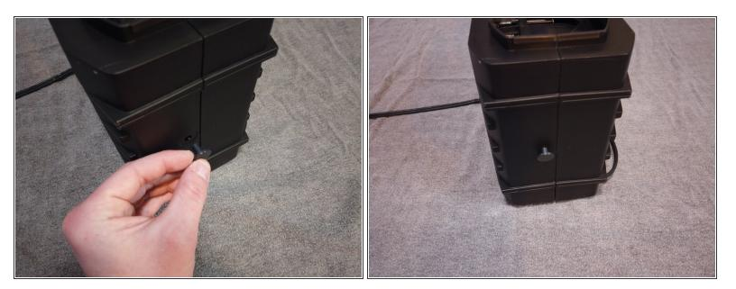
• Gently put the pressure plate back onto the pressure pin.
