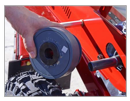
Remove the centrifugal clutch and shaft key from the spindle.
