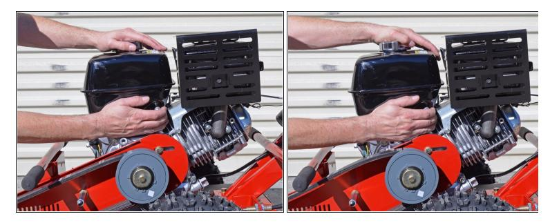
• Slide the engine towards the cutter blade to loosen the drive belt.
