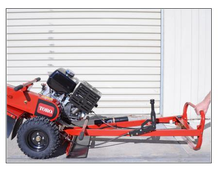
Tilt the machine so that it is resting on the handle with the cutter wheel raised.
