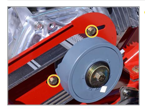
Use a 1/2 inch wrench to loosen the two bolts behind the centrifugal clutch enough to allow the motor to slide freely. Do not remove the bolts.
