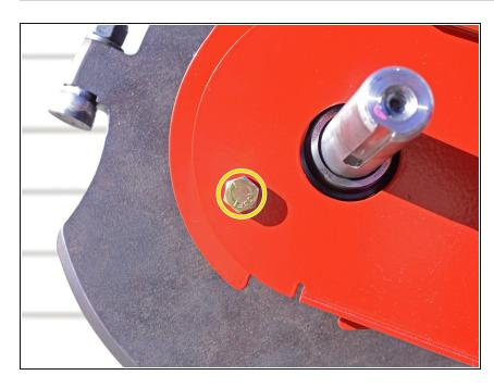
Use a 1/2 inch socket to remove the bolt next to the cutter wheel shaft securing the guard plate to the frame.
