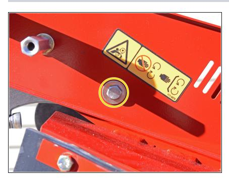
Use a 9/16 inch socket to remove the bolt and accompanying washer securing the guard plate to the frame.
