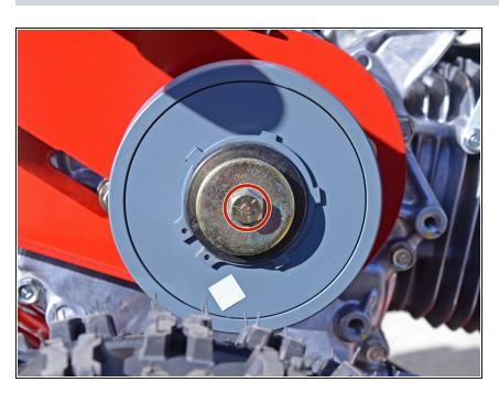
Use an impact wrench with a 9/16 inch socket to remove the bolt and washer securing the centrifugal clutch to the spindle.
