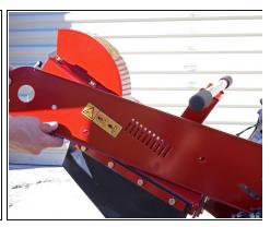
• Remove the guard plate from the frame.
