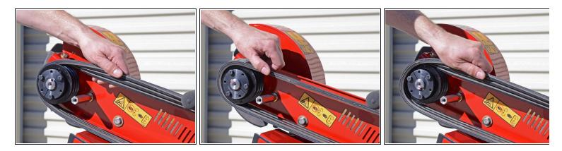
• Lift the drive belt up and away from the machine while rolling it towards the cutter head to gradually roll it off of the pulley.
