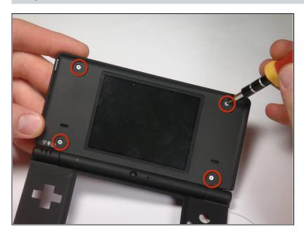
Remove 4 Phillips screws with a #00 Phillips screwdriver.
