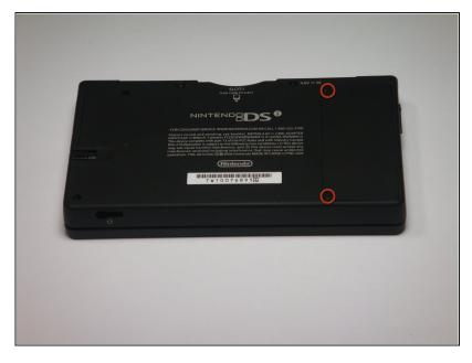
Loosen the two screws on the battery panel. Then lift the panel up to remove it.
