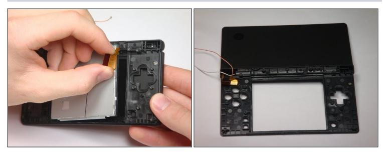
Flip the case open, and push the lower screen assembly out of the frame.
