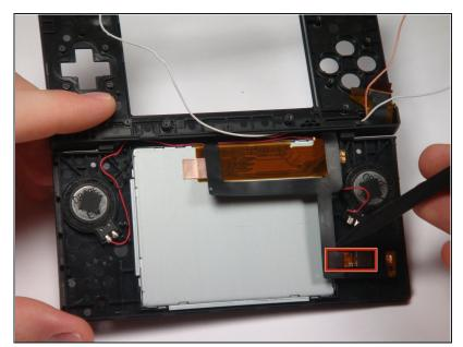
Use a spudger to pry the camera out of its place.
