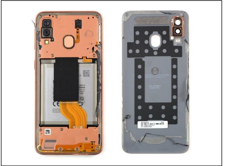
**⚠** To avoid tearing the fingerprint cable during the following step, make sure to gently press down the fingerprint reader while lifting the back cover.
