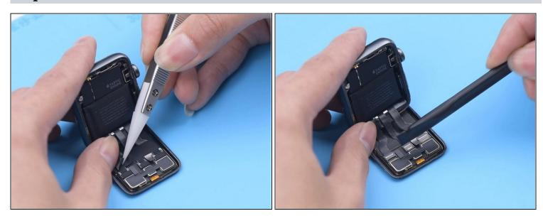
• Peel off the tape covering the display flex cables with <u>tweezers</u>. Please do not damage the flex cables while peeling off. Then disconnect the flex cables.
