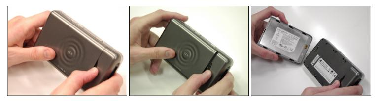
• Push the black button and slide the battery casing to the left simultaneously, until the battery is completely separated from the device.
