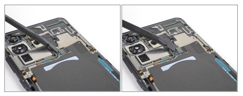
Use a spudger to pry up and disconnect the wireless charging coil connector.
