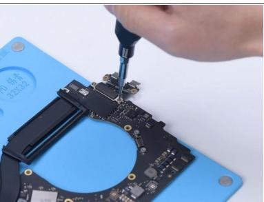
Then we remove the motherboard and install the power connector flex cable.
