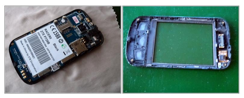
Now using the flathead screwdriver, prise the plastic that makes up the front, away from the circuit board. Like the back piece, it has a series of clips around the edge, and should lift free without much effort.
