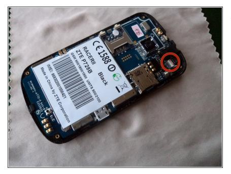
Carefully remove the ribbon cable that connects the capacitive screen to the main board. You need to carefully lift the small tab, then pull the cable out.
