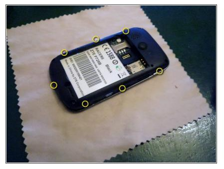
Using a flathead screwdriver, carefully prise the black plastic away. It's held in with a series of clips, and should come away easily.
